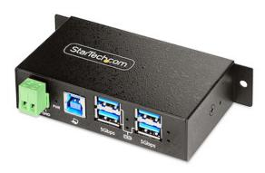
This 4-port Managed Industrial USB 3.2 Gen 1 (5Gbps) Hub enables users to toggle individual USB ports on/off and to reboot the hub, using the USB Hub Administrator Software (free to download). With robust housing and versatile power input options, the USB Hub is designed to cater to the needs of IT Professionals working in industrial settings such as factories, warehouses, offices, and other similar environments.
